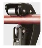
**Tube Capacity** 1/8" ~ 1-5/8" (3 MM ~ 41 MM)
