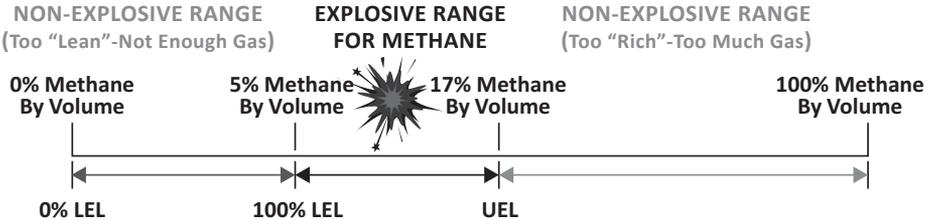
**BELOW** a specific LEL for a combustible gas, the air/gas mixture is too “lean” (not enough gas is present to burn). See the above visual diagram that applies to Methane only.
